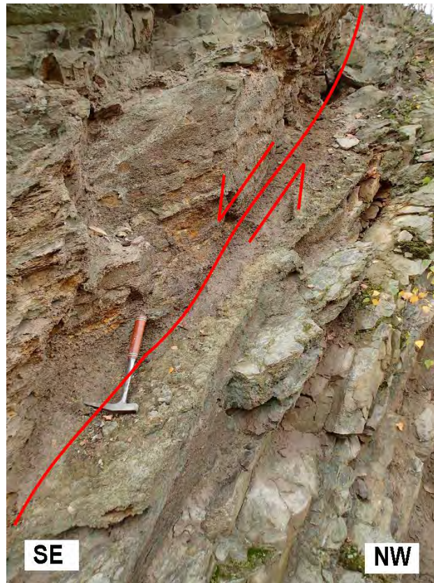
Fig. 1: View of the mylonite subzone normal fault plane D 104/40 at Rančířov quarry. Photo L. Daňková 2014.
