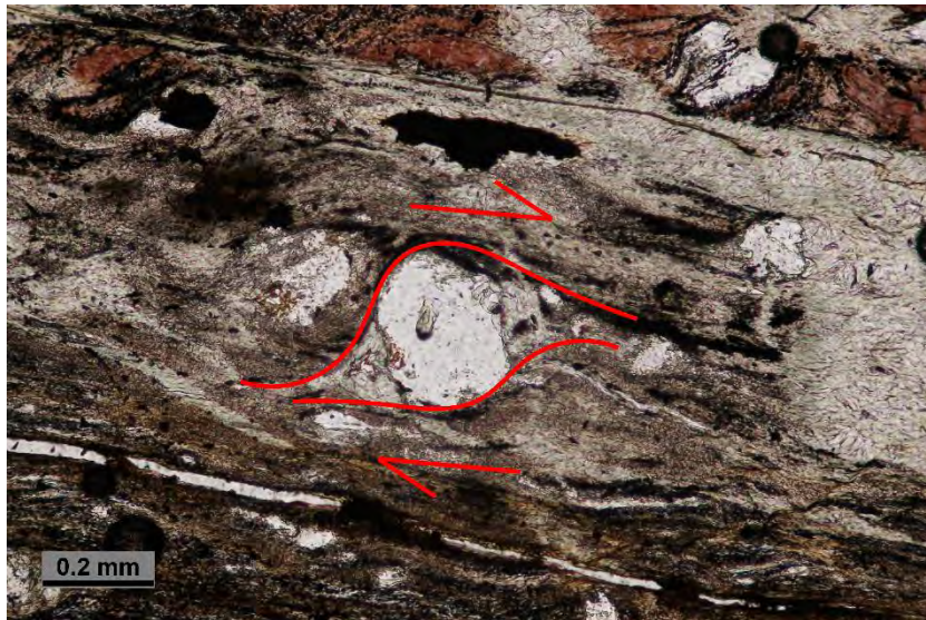
Fig. 2: The \sigma -porphyroblast of plagioclase as the kinematic indicator at the thin section of mylonite from Rančívov quarry. Photo L. Daňková 2014.
