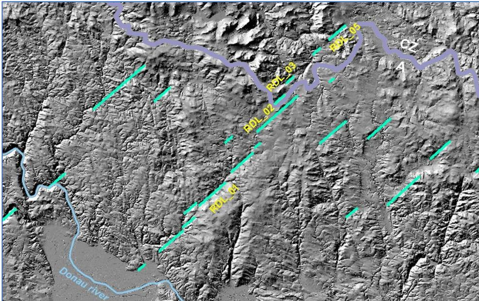
Fig. 1: Topo-lineaments related to the Rodl fault zone.
