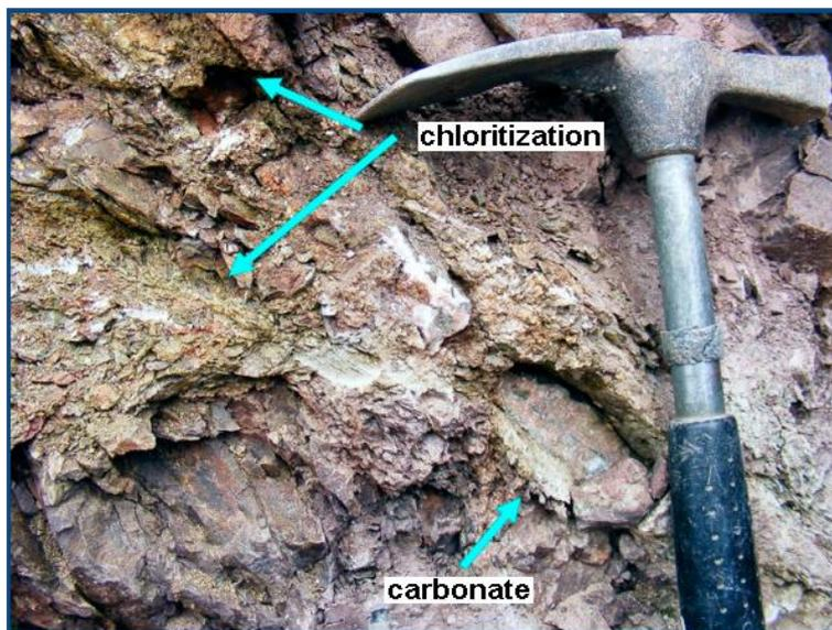
Fig. 4: Tectonically affected and altered Permian siltstones dusters in the zone of Drahotěšice fault with carbonate veins and crushed zones with chlorite. Úsilné, R-V trench. Photo I. Prachař, 2009.
