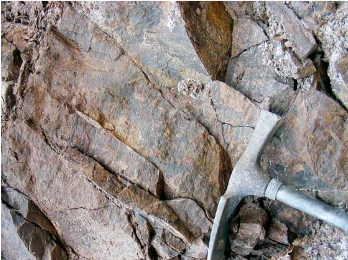
Fig. 8: Detail view of the wall of the R-V trench with exposed Permian siltstones with slickensides and oblique striations on the divisional planes. Photo I. Prachař, 2009.
