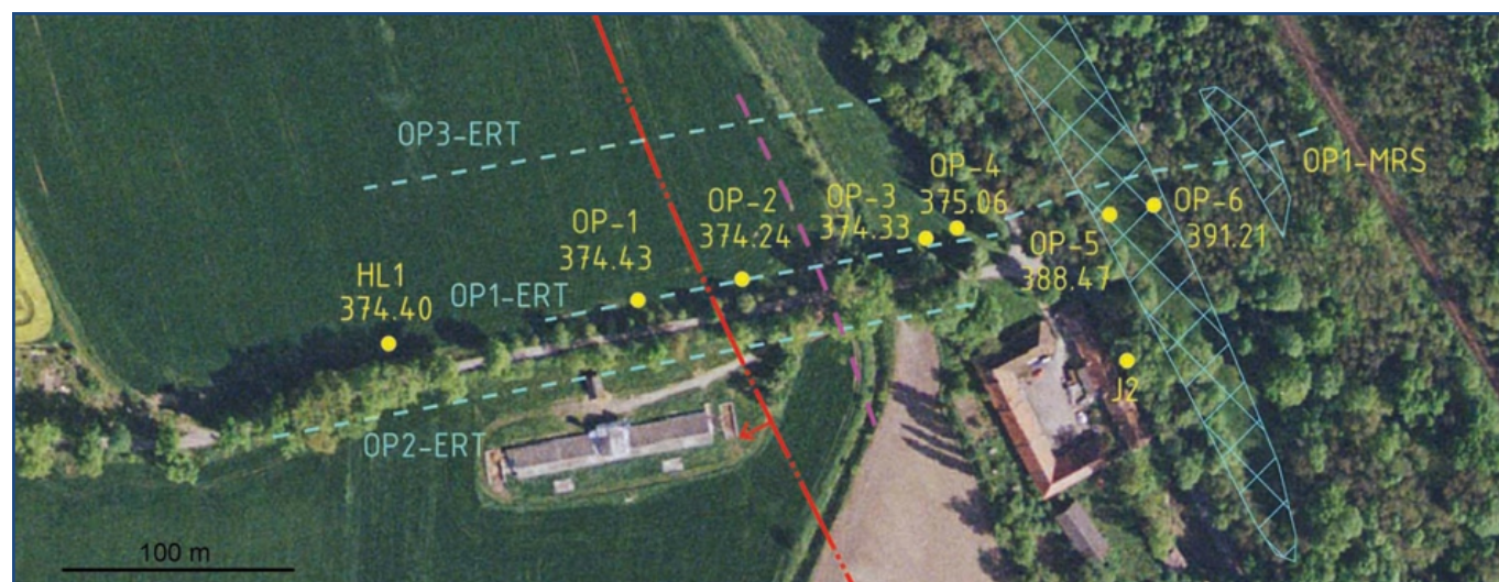
Fig. 10: Situation on the “Opatovice profile”. Light blue dotted lines - geophysical profiles with the name and the method used. Core boreholes are marked in yellow (name and altitude). Light blue hatch - platforms with clastic sediments. Red dash-and-dot line - supposed line of Hluboká fault covered by Pleistocene sediments of the Vltava River. Purple dashed line - supposed boundary between kaolinized crystalline rock and sound rock. Adopted from ŠPAČEK ET AL., 2010.
